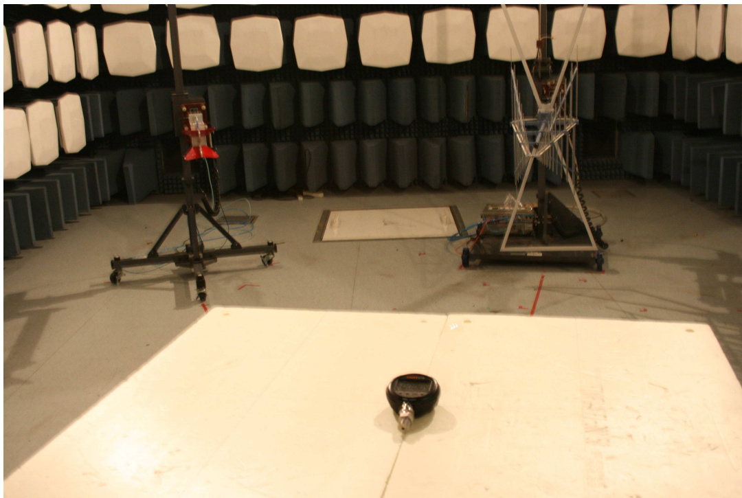
Photograph 1: Set-up for Spurious Emissions, below 1GHz
