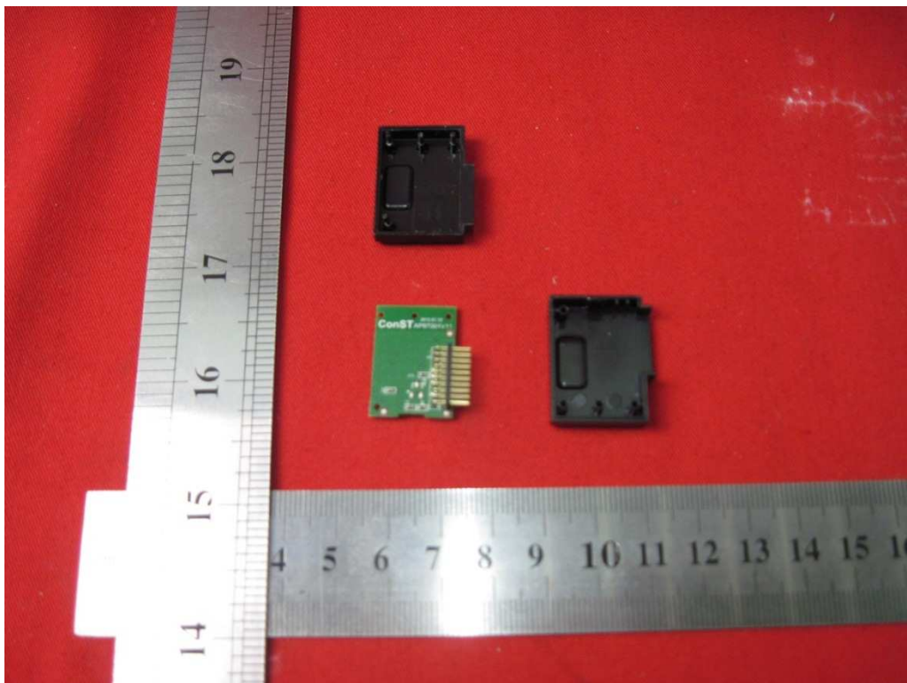
Internal of wireless module
