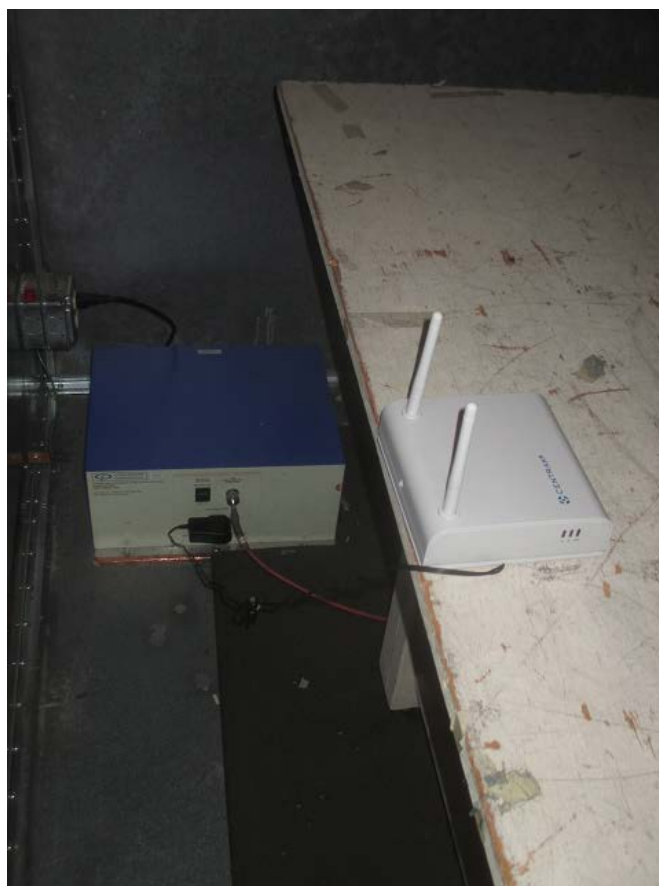
Figure 2 Conducted Emission Test Setup
