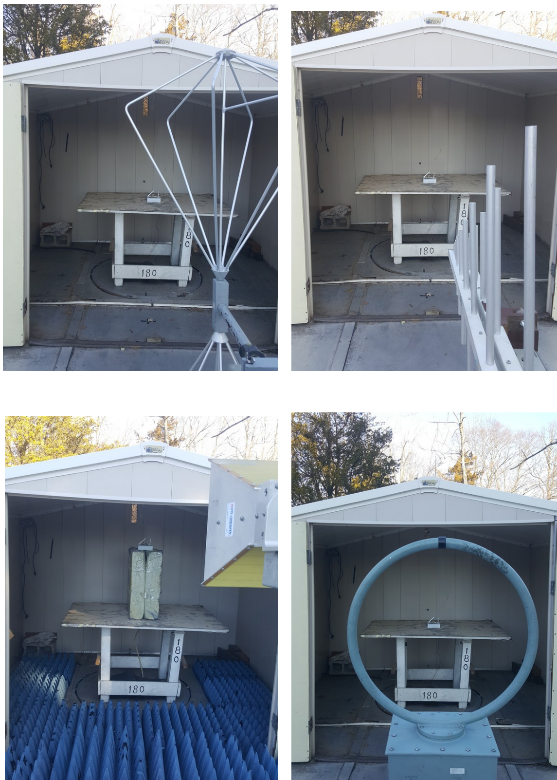
Figure 1 EUT Configuration for Radiated Emission Tests
