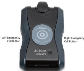
This action Awakens Elpas Wi-Fi Man Down Tag from Sleep Mode and also enrolls its unique factory installed **ID Number** (a six-digit hexadecimal value) into the Host RTLS Application.
