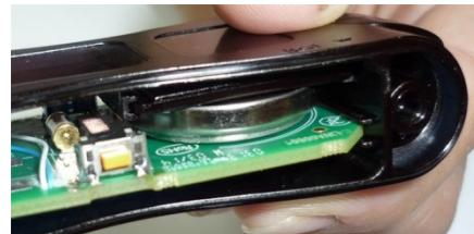
3. **First time replacement:** Utilize the pull tab (find it with the **Bat▼** mark engraved on the back) to slide the battery out of the Transmitter.
