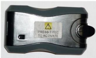
1. Prior to initial usage, remove the Activation Label and simultaneously press, both of the emergency call push buttons for at least 7 seconds.
