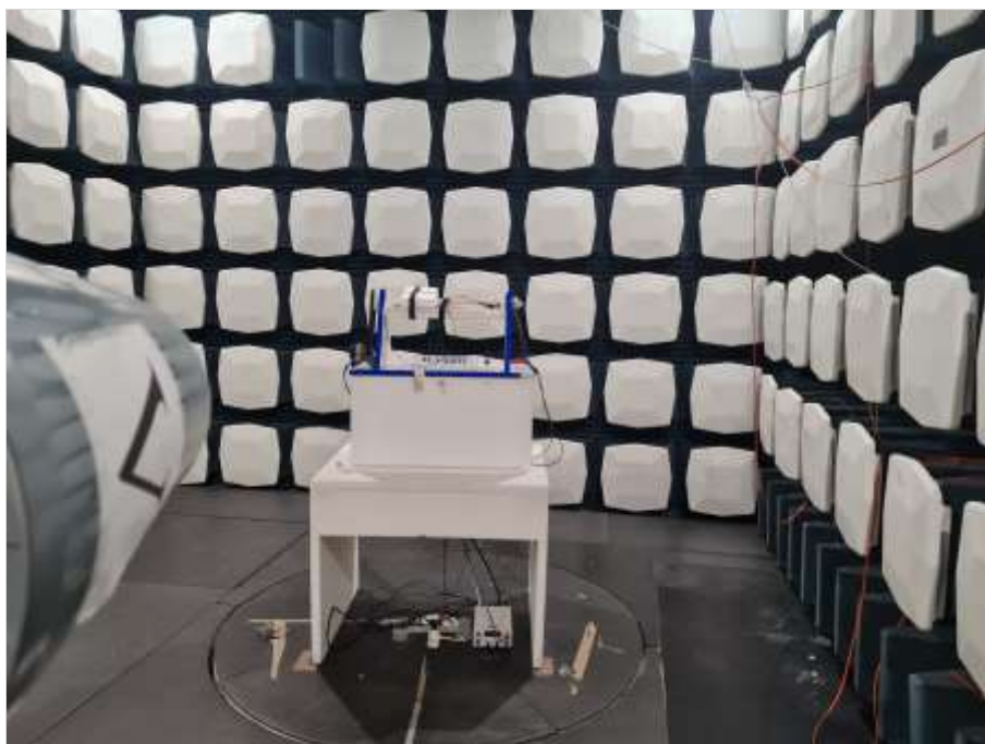
Photograph 2: EUT test setup in the fully anechoic chamber, overview_EUT elevation 0°
