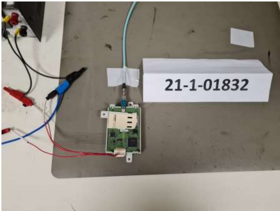
Photograph 9: EUT setup conducted measurement, close up view
