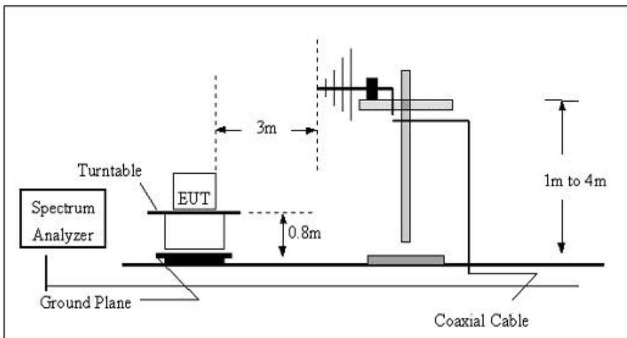
**Radiated Emission Test Set-Up, Frequency Over 1GHz**
