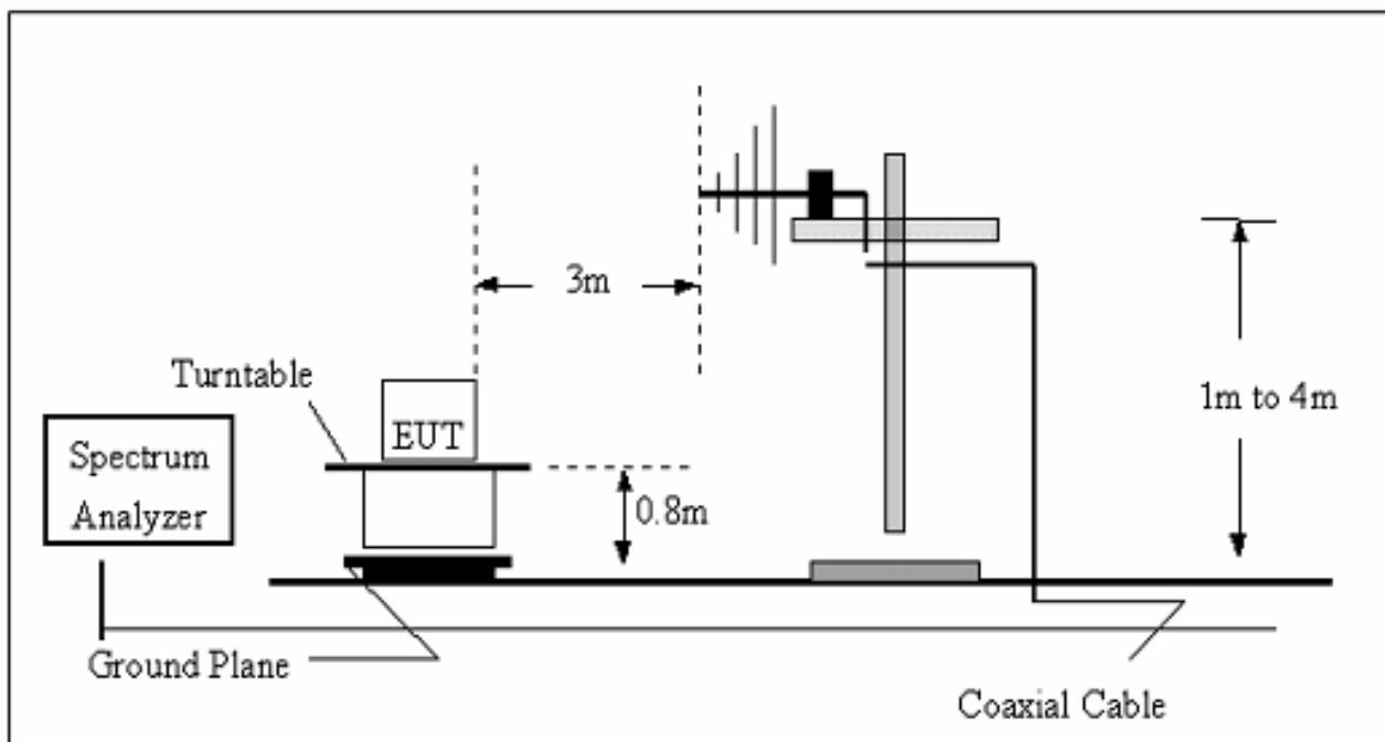
**Radiated Emission Test Set-Up, Frequency Over 1GHz**
