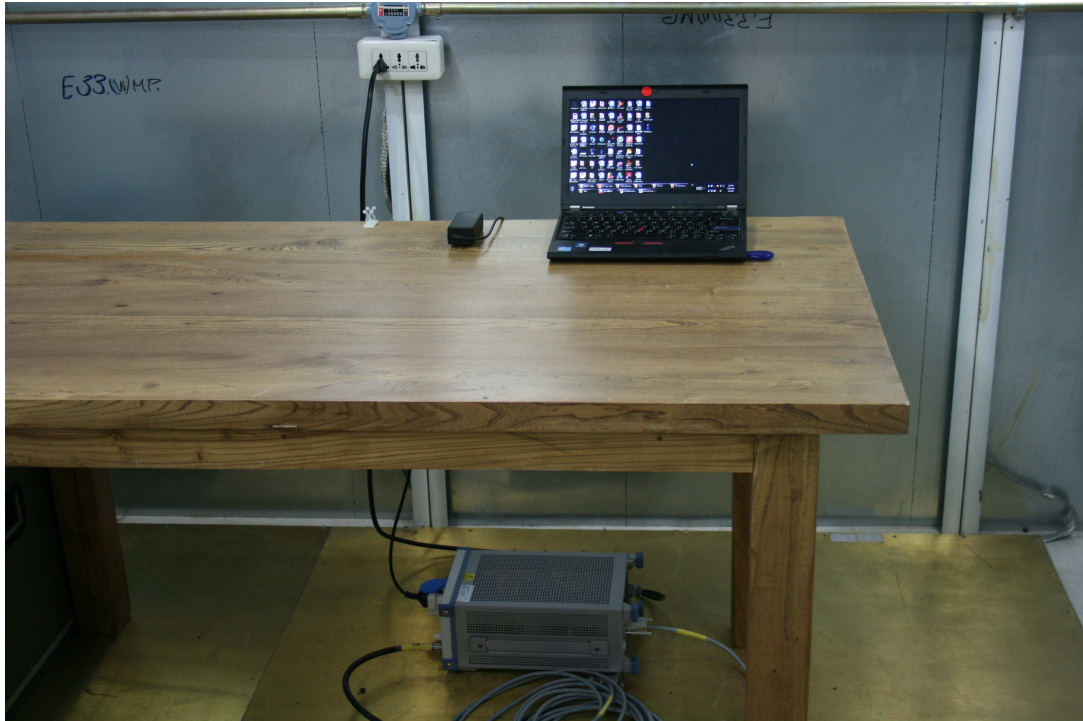
Photograph 3: Set-up for Conduited emission
