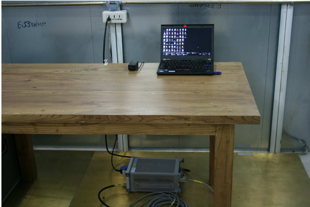
Photograph 3: Set-up for Conduited emission
