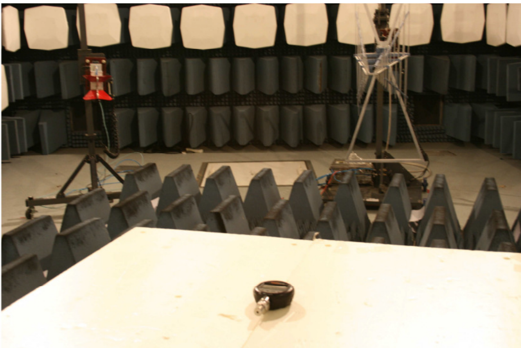
Photograph 2: Set-up for Spurious Emissions, above 1GHz
