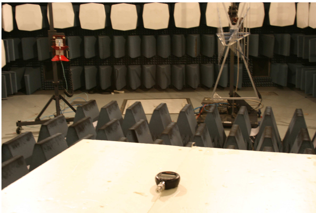
Photograph 2: Set-up for Spurious Emissions, above 1GHz
