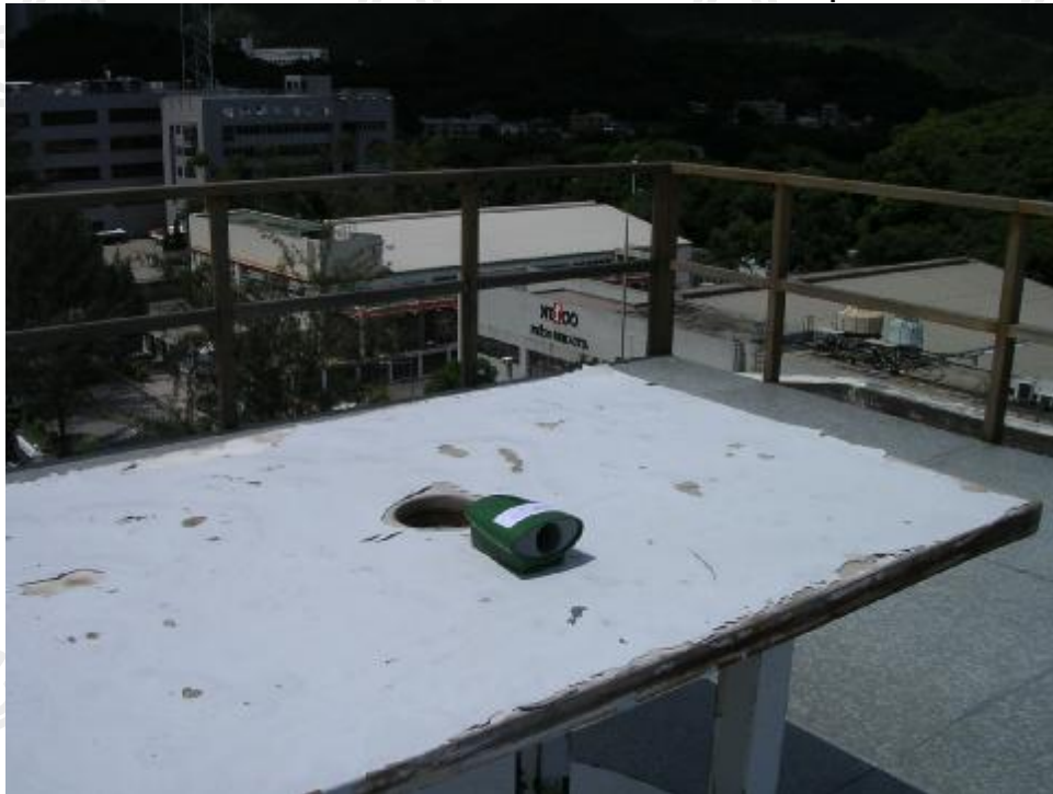
Measurement of Radiated Emission Test Set Up
