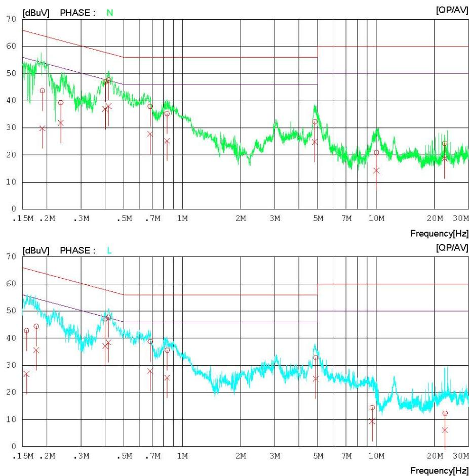
**AC Line Conducted Emissions (List) & Modulation: GFSK**
