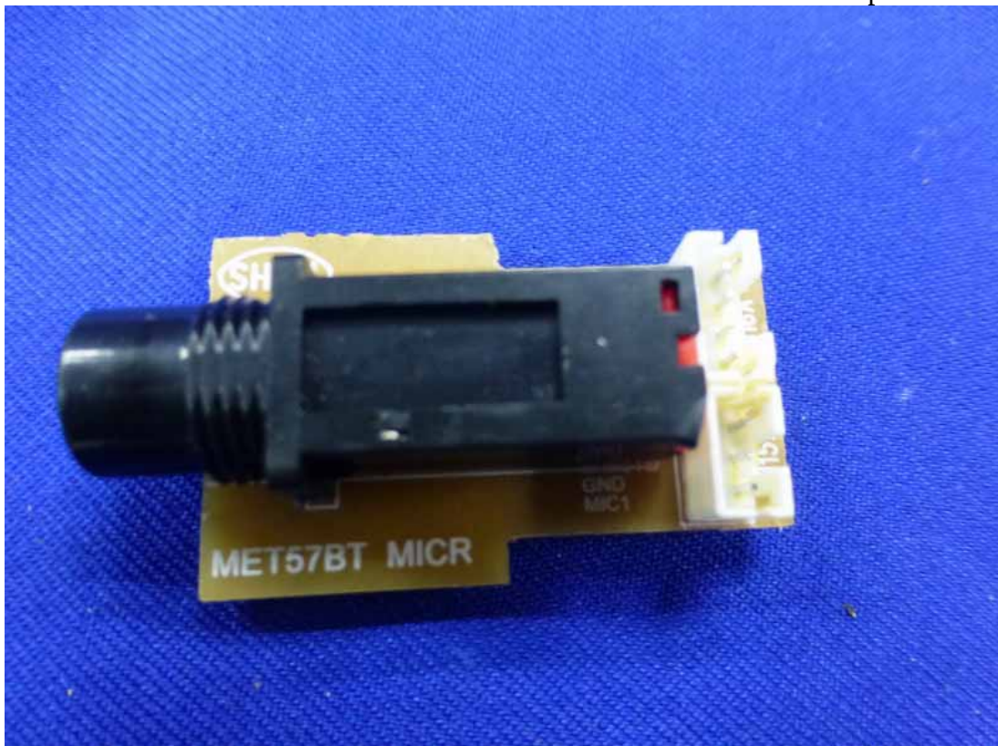
Figure 28 Component side of the PCB
