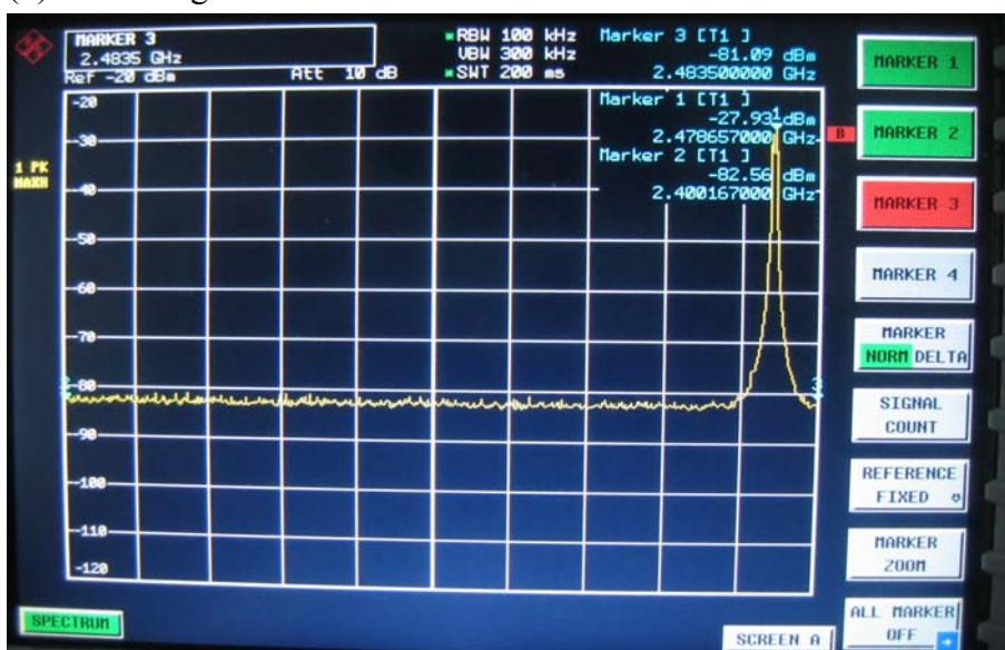
The test result for the Emissions radiated outside of the specified frequency bands , please refer the section 5.3.1 of this report.
