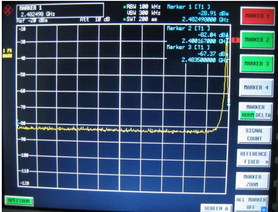
The test result for the Emissions radiated outside of the specified frequency bands , please refer the section 5.3.1 of this report.
