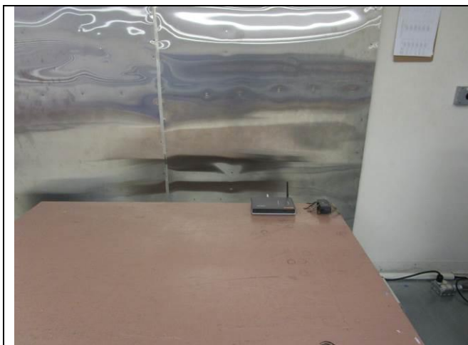
Conducted Emission test setup– Front View
