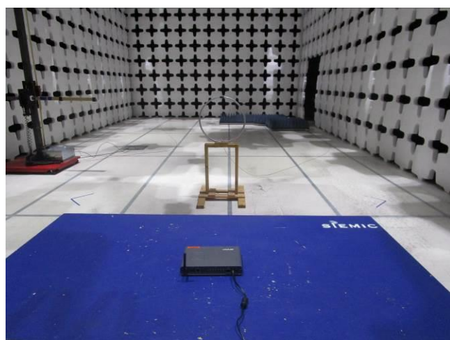
R Emission Test setup (<30MHz) – Rear View 0 deg
