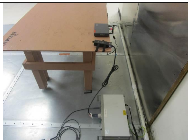
Conducted Emission Test setup – Rear View
