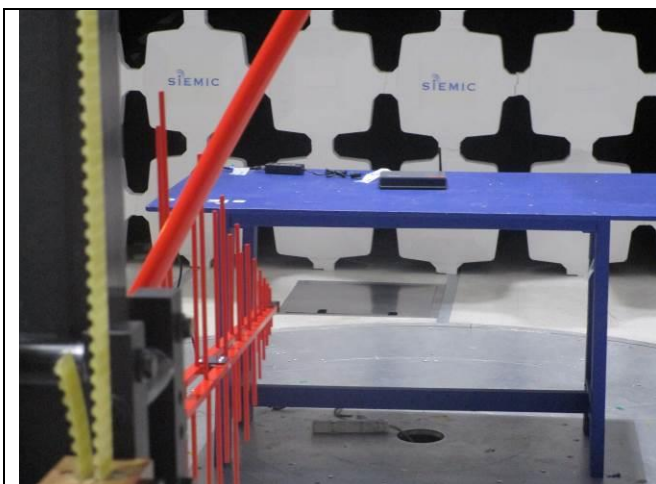
Radiated Emission Test setup (<1GHz) – Front View
