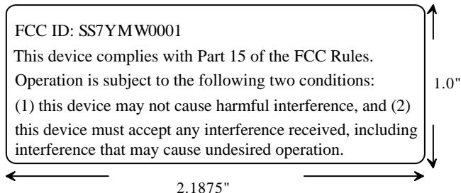
Specifications: Text is black in color and is left justified. Labels are printed in indelible ink on permanent adhesive backing and shall be affixed at a conspicuous location on the EUT.
