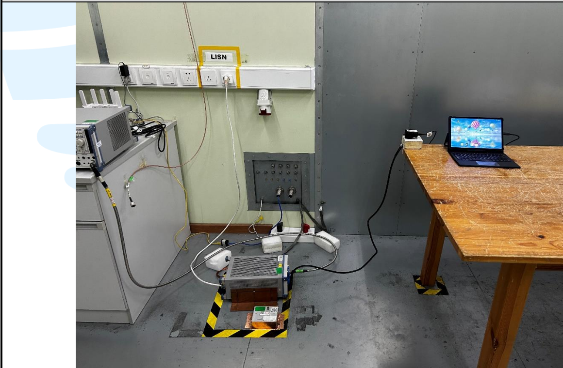
Conducted Emission Test Setup
