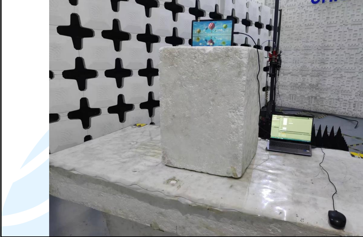
Radiated emission Test Setup (Above 1 GHz)
