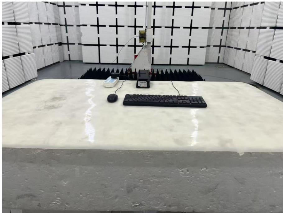
**Model: SP60****Set-up for Conducted Emission on AC Mains (CE)**
