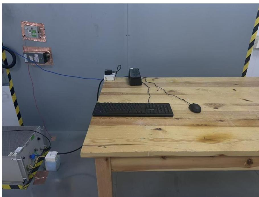
**Set-up for Radiated Emission (RE), Below 1GHz**
