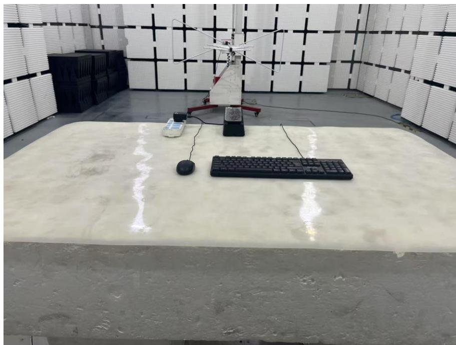
**Set-up for Radiated Emission (RE), Above 1GHz**
