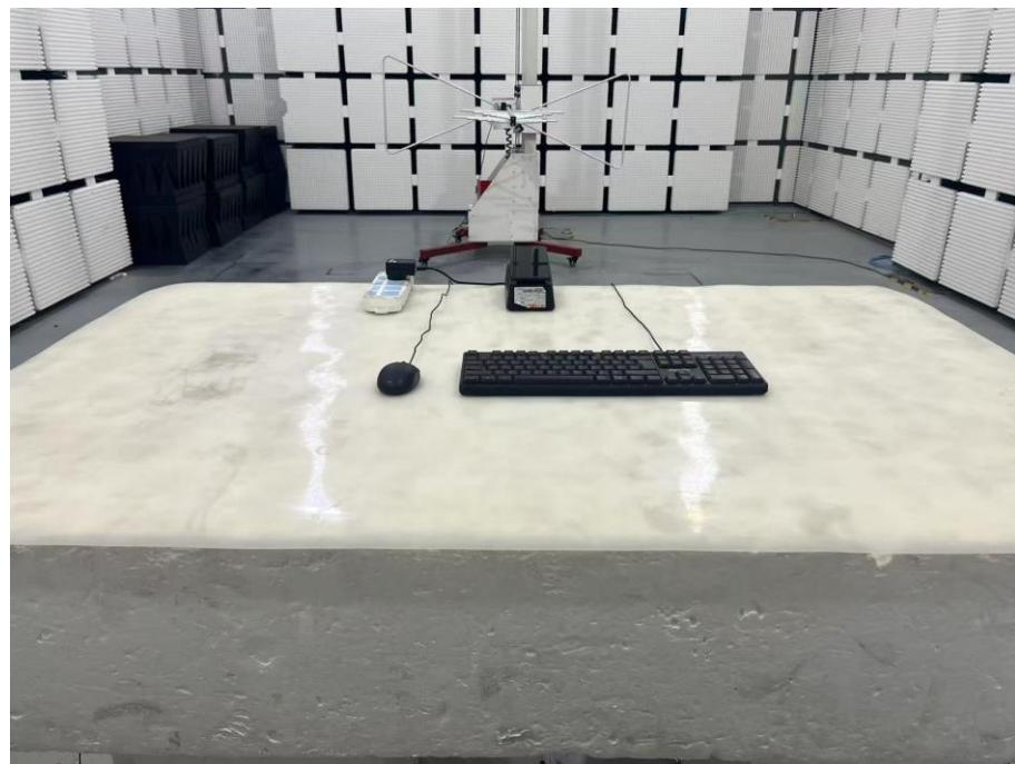
**Set-up for Radiated Emission (RE), Above 1GHz**
