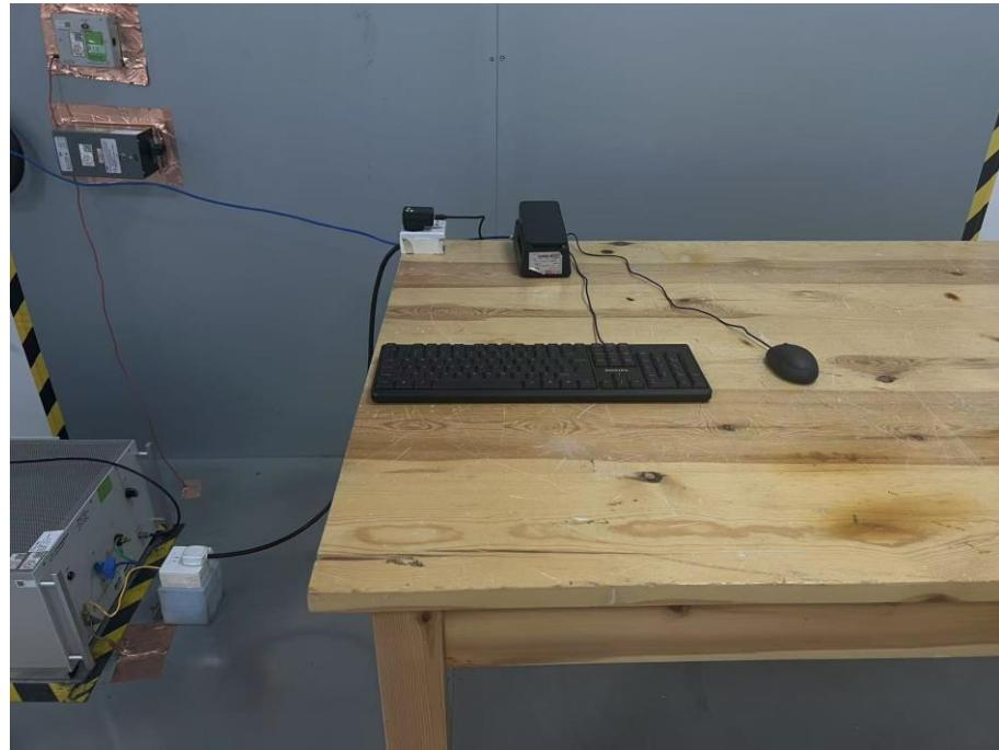
**Set-up for Radiated Emission (RE), Below 1GHz**
