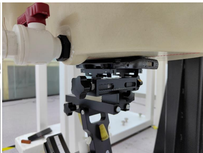
Fig-4.15 Rear Face of EUT with 0 cm Gap (Extremity Mode)
