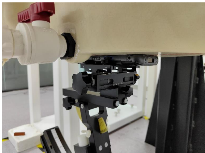
Fig-4.14 Front Face of EUT with 0 cm Gap (Extremity Mode)
