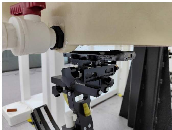
Fig-4.10 Rear Face of EUT with 1 cm Gap (Body-Worn Mode)
