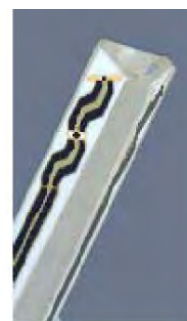
Figure E.2.2 Probe Thick-Film Technique
