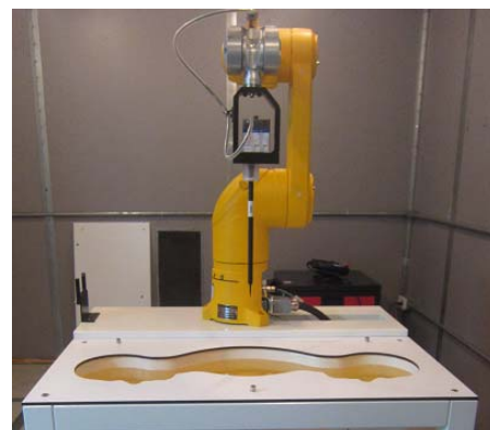
Figure 4.1 DASY5 Test System
