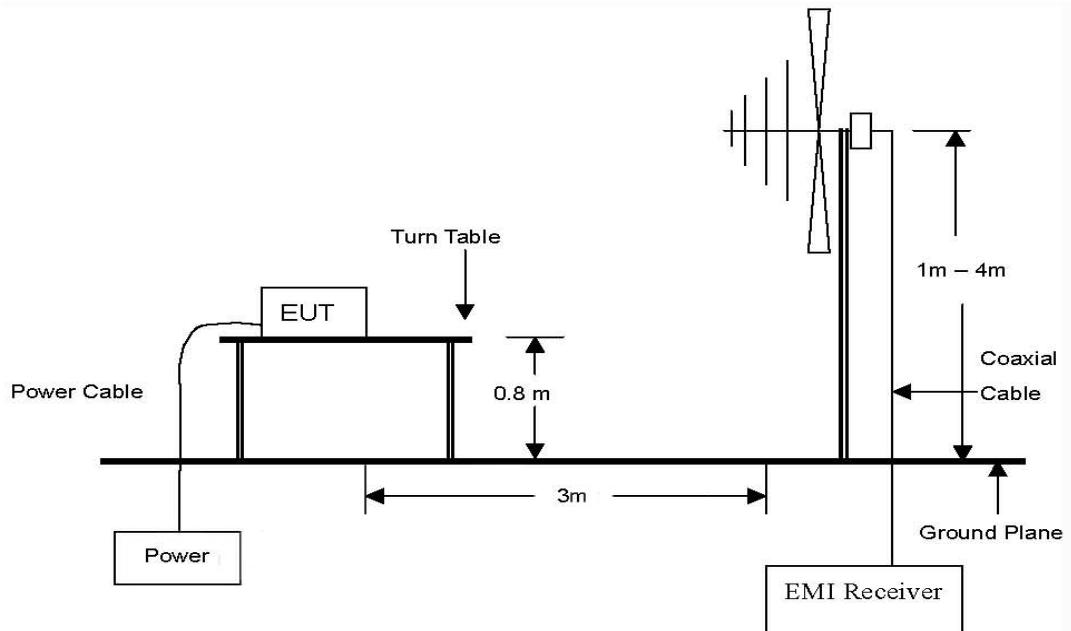
The diagram below shows the test setup that is utilized to make the measurements for emission from 1 GHz to 24 GHz Emissions.
