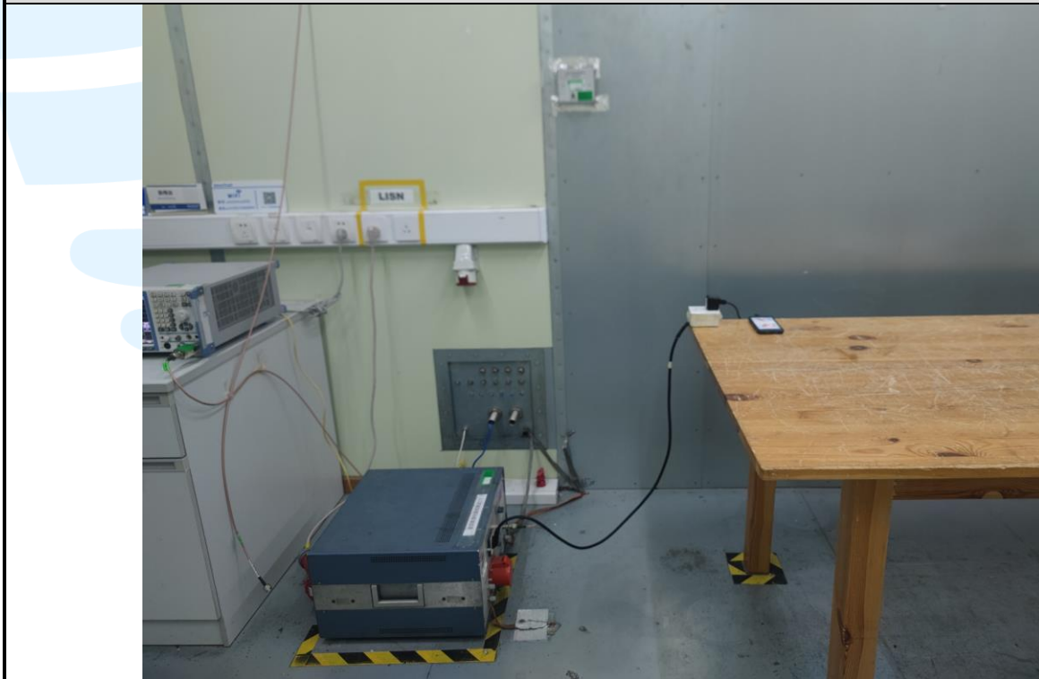
Conducted Emission Test Setup
