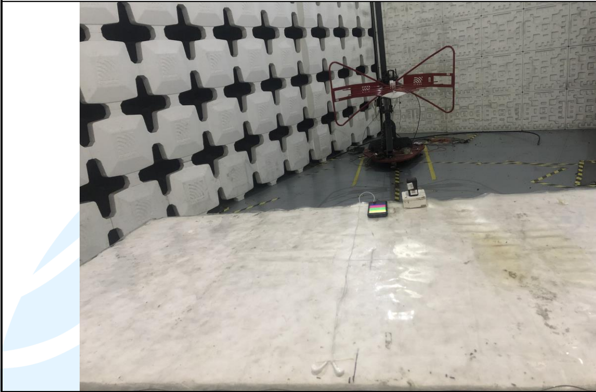
Radiated emission Test Setup-1 (30 MHz~1 GHz)
