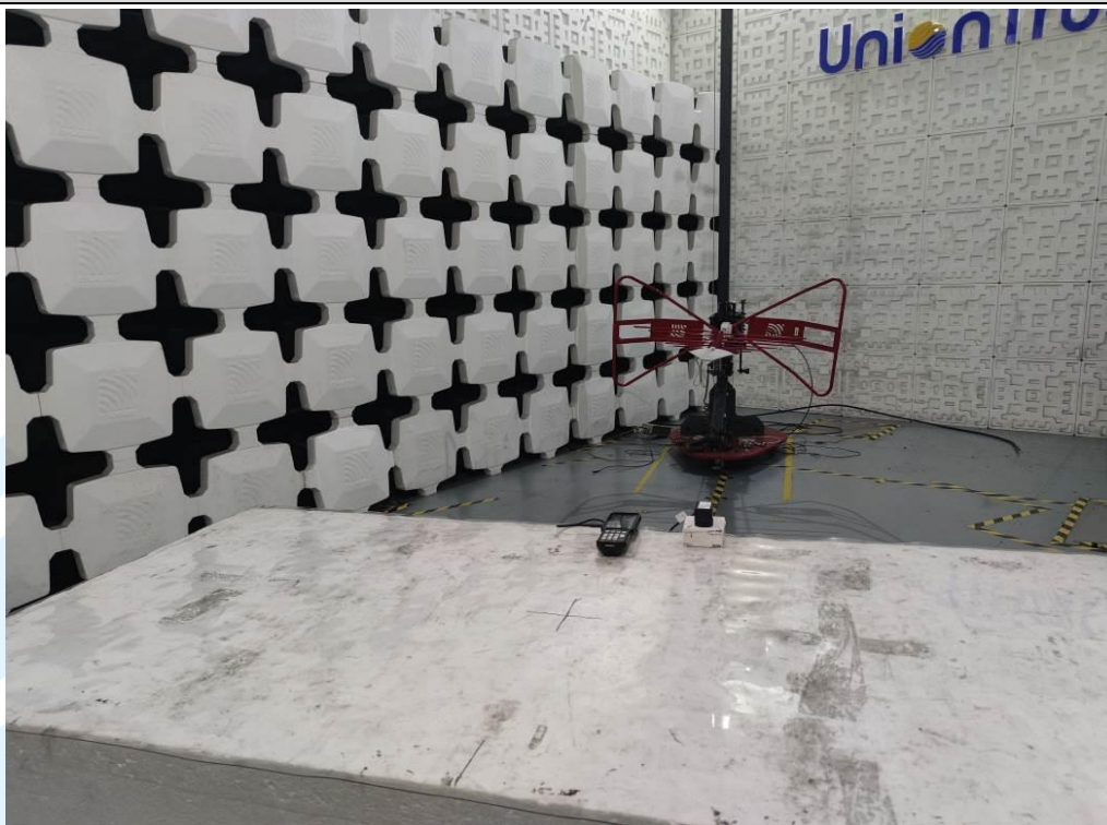
Radiated emission Test Setup-1 (30 MHz~1 GHz) – Test Mode 3
