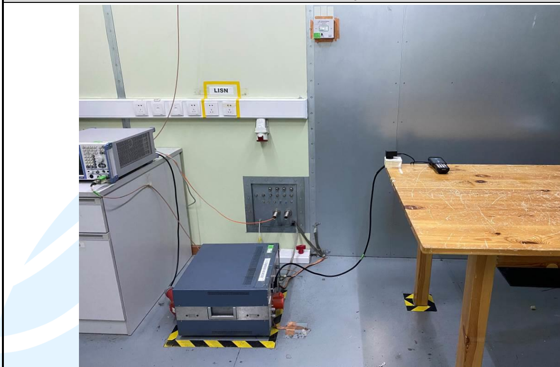
Conducted Emission Test Setup-3 – Test Mode 2&4
