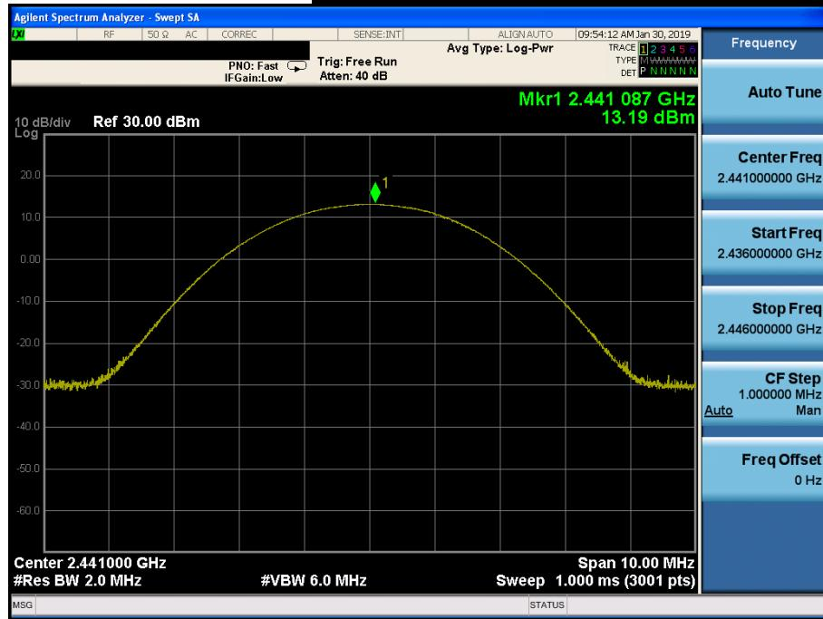
**Peak Output Power****Highest Channel & Modulation : 8DPSK**
