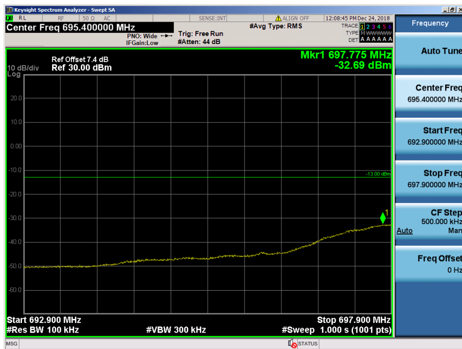
LTE Band 12 / 3MHz / QPSK - RB Size/Offset (15/0)
