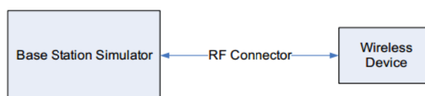
Figure 10.1 Power Measurement Setup
