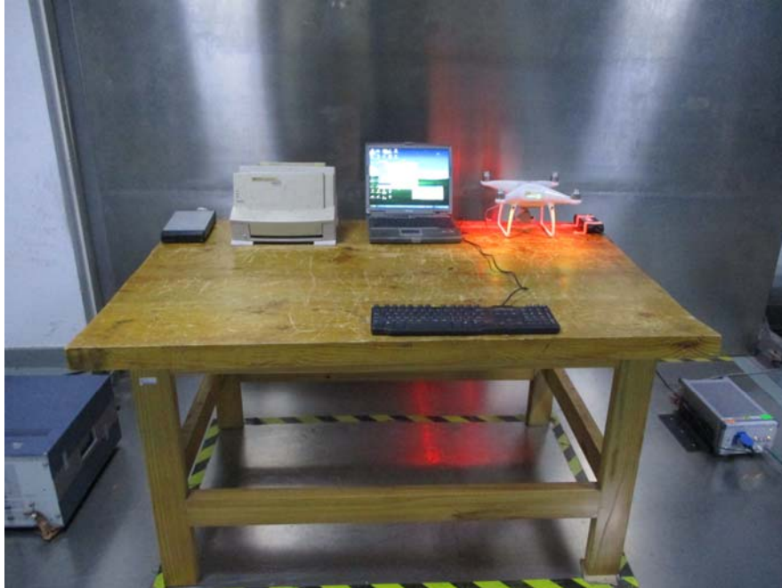
Conducted Emissions – Front View(Downloading)
