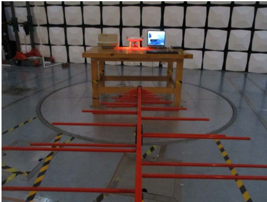
Radiated Emission Downloading Front View (Below 1GHz)
