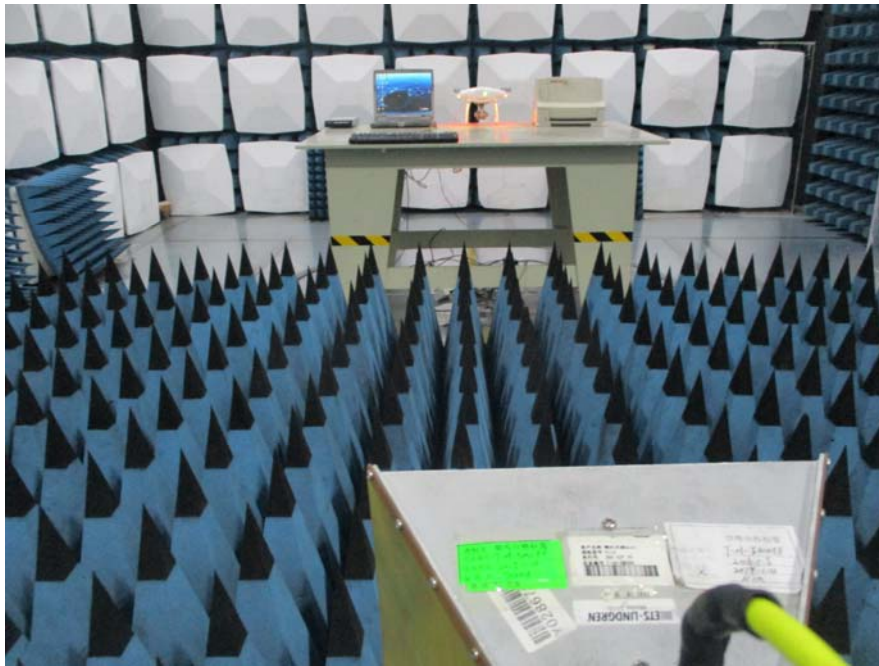
Radiated Emission Downloading Front View (Above 1GHz)
