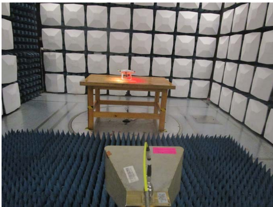
Radiated Emission Operation View (Above 1GHz)
