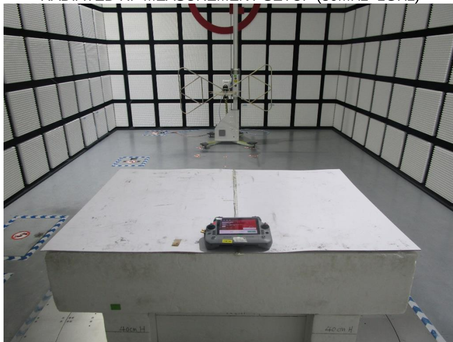
RADIATED RF MEASUREMENT SETUP (Below 30MHz)
