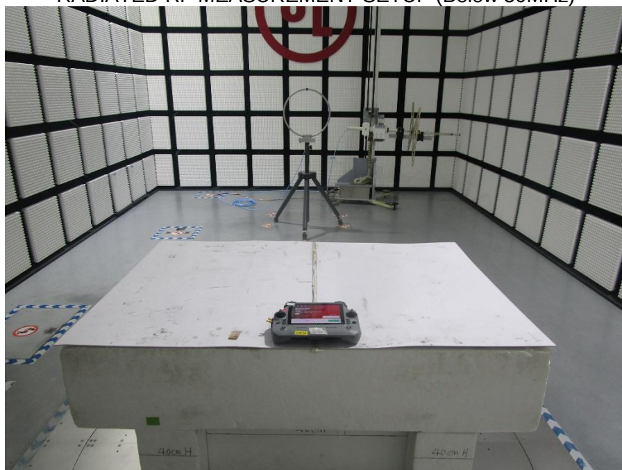
RADIATED RF MEASUREMENT SETUP (Below 30MHz)
