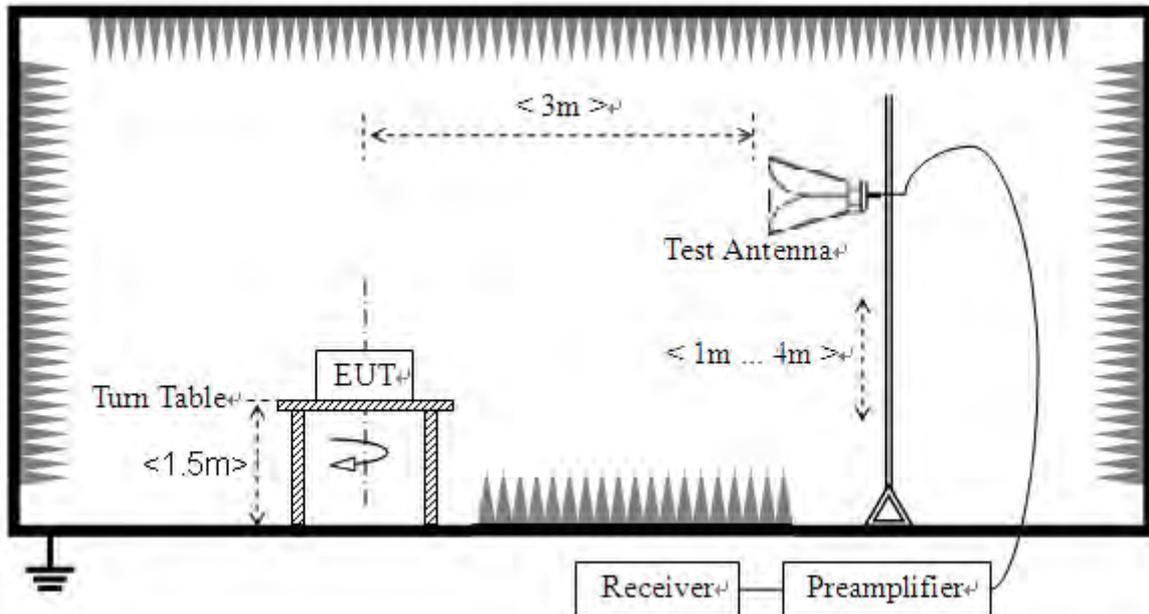
The test site semi-anechoic chamber has met the requirement of NSA tolerance 4dB according to the standards: ANSI C63.4-2014. For radiated emissions below or equal to 1GHz, The EUT was set-up on insulator 80cm above the Ground Plane, For radiated emissions above 1GHz, The EUT was set-up on insulator 150cm above the Ground Plane. The set-up and test methods were according to ANSI C63.10-2013.
