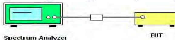
The EUT (Equipment under the test) which is powered by the Battery is coupled to the Spectrum analyzer; the RF load attached to the EUT antenna terminal is 50Ohm; the path loss as the factor is calibrated to correct the reading, all test result in Spectrum analyzer.
