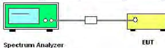
The EUT which is powered by the battery, is coupled to the Spectrum Analyzer; the RF load attached to the EUT antenna terminal is 50Ohm; the path loss as the factor is calibrated to correct the reading.
