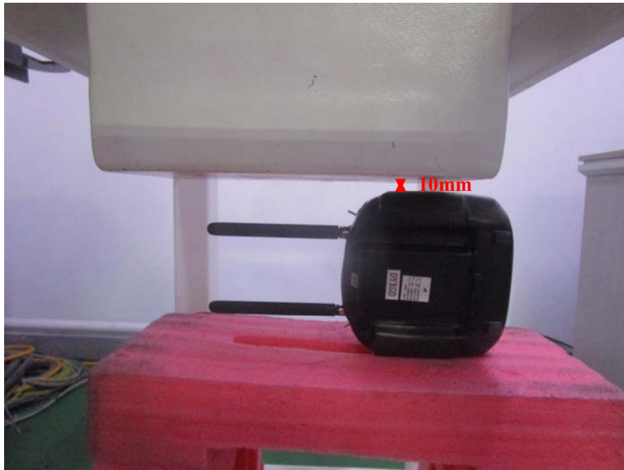
Test Position_Left (10mm)
