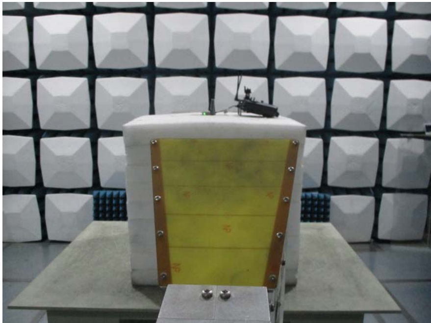
Radiated Emission Above 1GHz View
