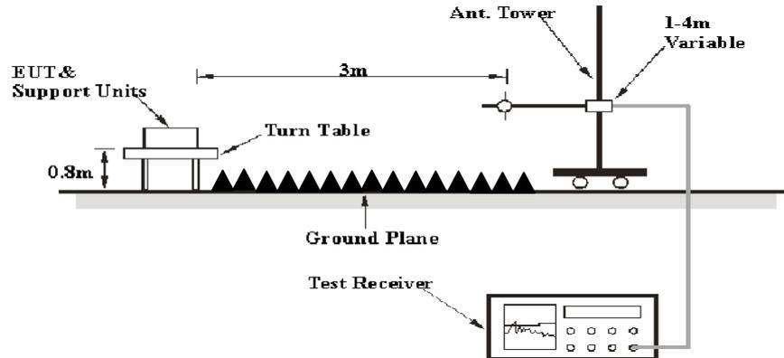
The radiated emission tests were performed in the 3 meters chamber test site, using the setup accordance with the ANSI C63.4-2009. The specification used was the FCC 15.209, and FCC 15.247 limits.
