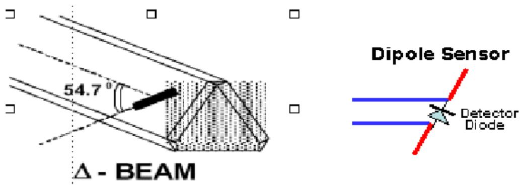
SAR is assessed with a calibrated probe which moves at a default height of 5mm from the center of the diode, which is mounted to the sensor, to the phantom surface (in the Z Axis). The 5mm offset height has been selected so as to minimize any resultant boundary effect due to the probe being in close proximity to the phantom surface.
