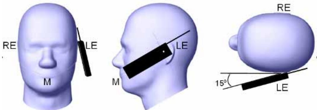
**Test positions for body-worn and other configurations**
