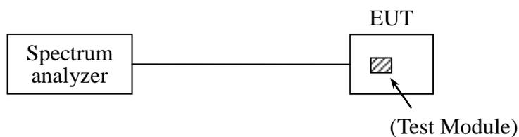
The measured output power was calculated by the reading of the spectrum analyzer and calibration.
