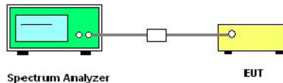
The EUT which is powered by the Battery, is coupled to the Spectrum Analyzer; the RF load attached to the EUT antenna terminal is 50Ohm; the path loss as the factor is calibrated to correct the reading.
