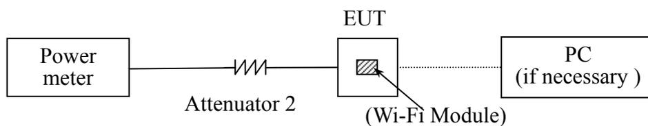
The EUT (Equipment under the test) which is powered by the Battery is coupled to the Power Meter; the RF load attached to the EUT antenna terminal is 50Ohm; the path loss as the factor is calibrated to correct the reading, all test result in power meter.
