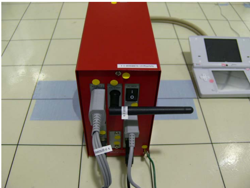
Photograph 3: Set-up for Radiated Emission, EUT Configuration Y-Axis
