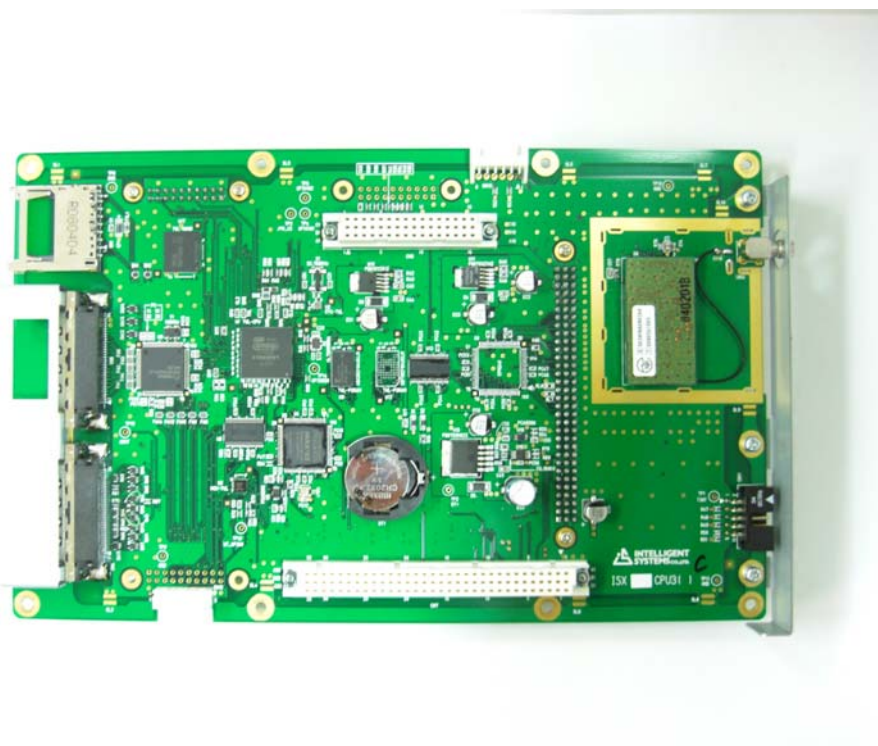
Top View CPU board without the shield and radio location
