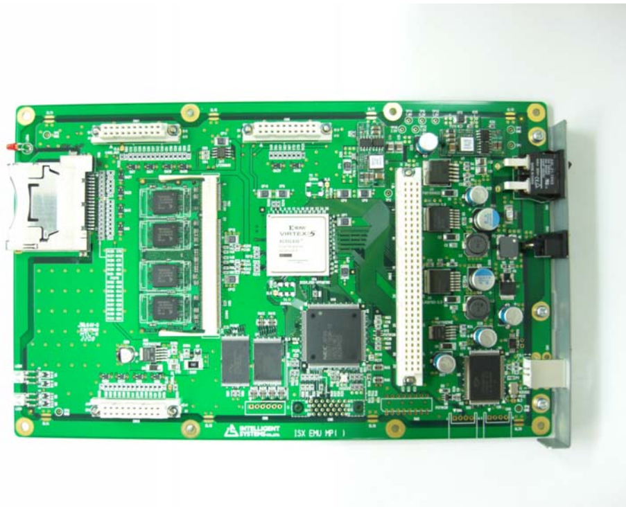
Top View Power Board
