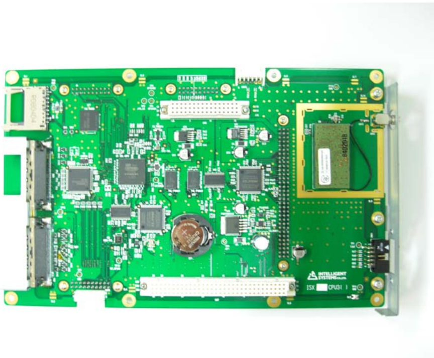
Top View CPU board without the shield and radio location
