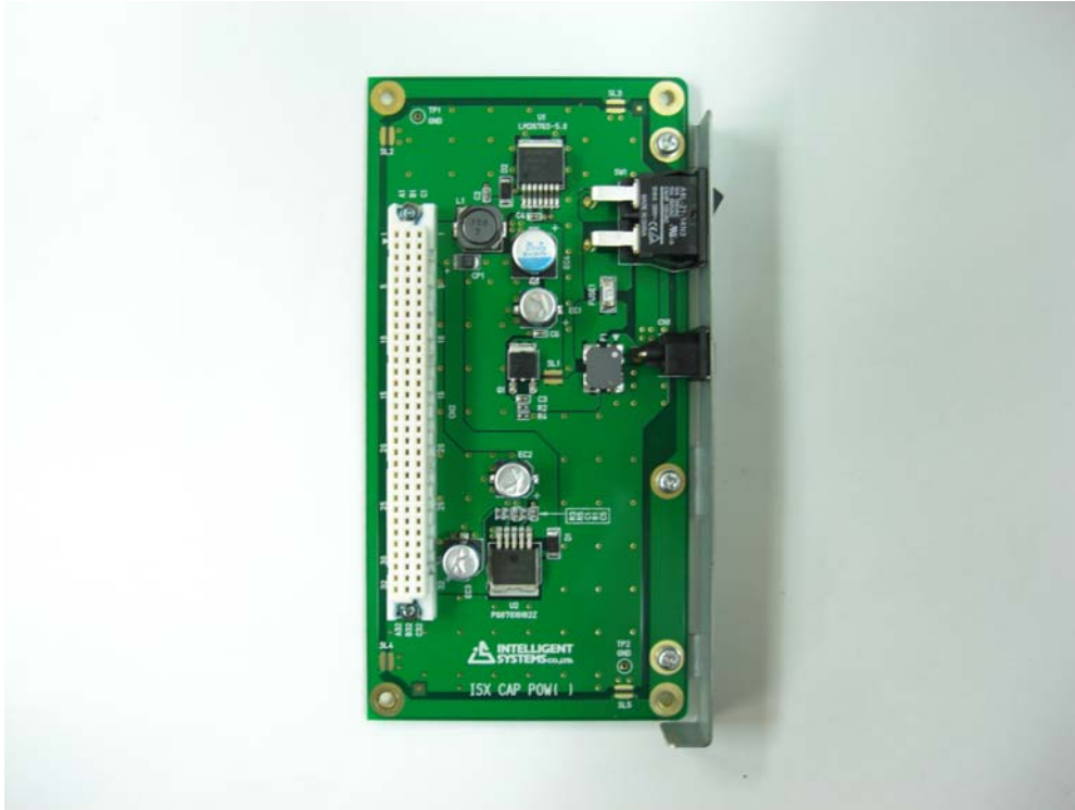
Top View Power Board
