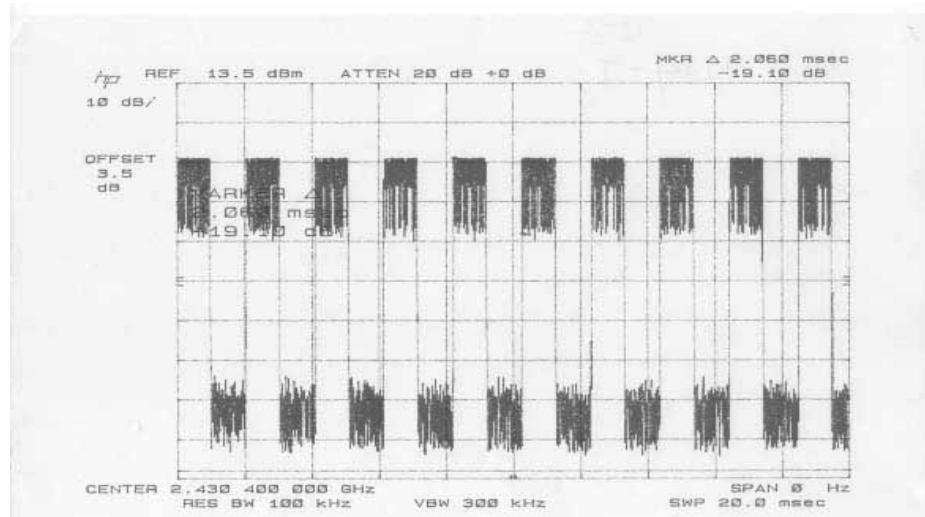
$$\text{Duty cycle value} = 20\log(T\text{width}/T\text{period}) = 20\log(980*10^{-8}/2.060*10^{-3}) = -6.45$$
