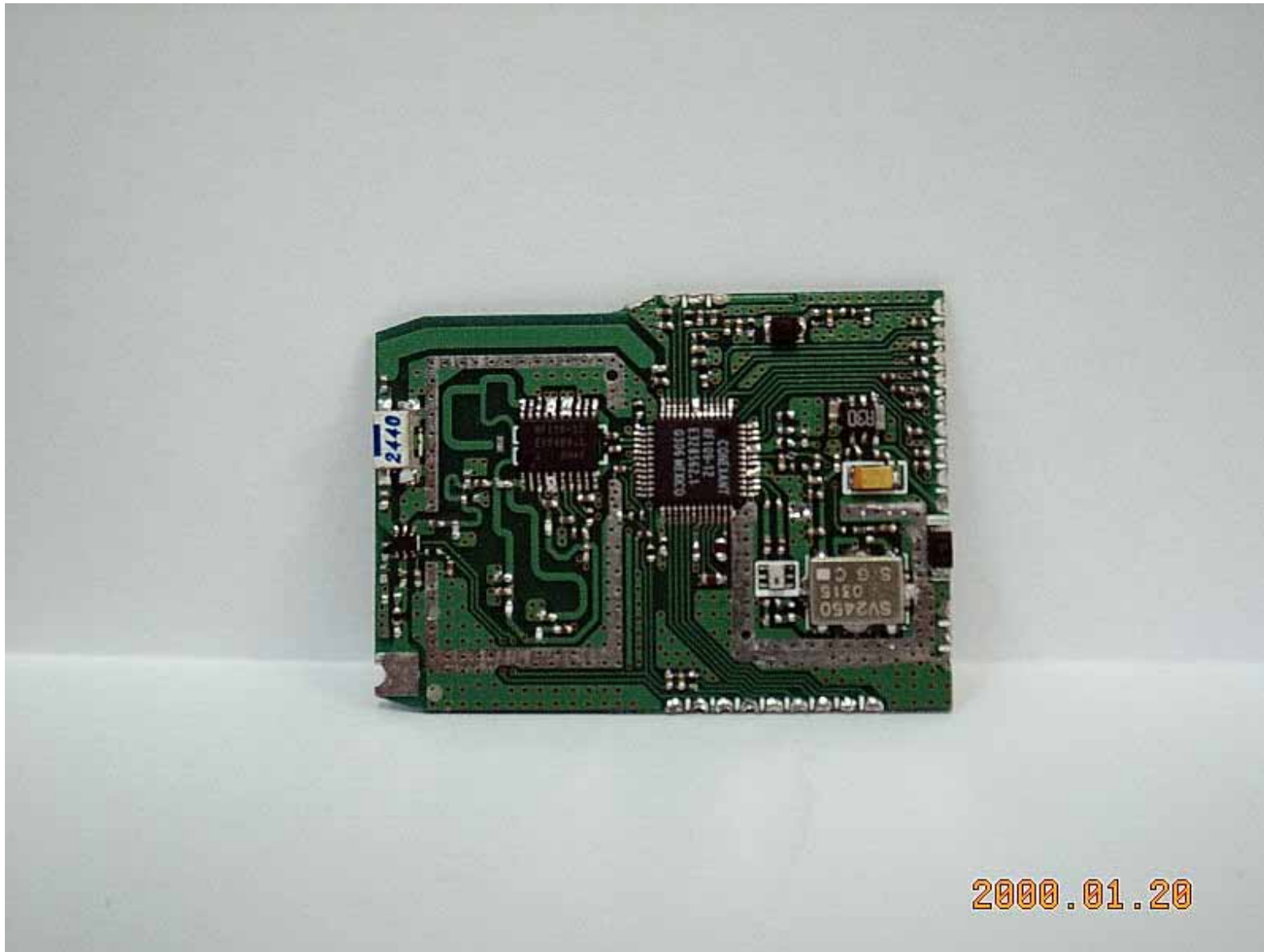
kt-24 rf pcb top (800x600x16M jpeg)
