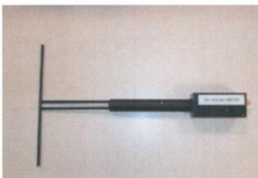
Figure 1 – Satimo COMOSAR Validation Dipole
