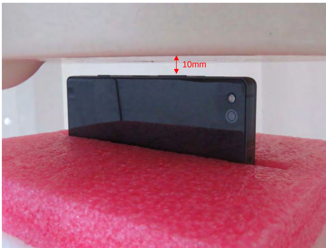
Picture 22: Left Side, the distance from handset to the bottom of the Phantom is 10mm For Single Screen Mode
