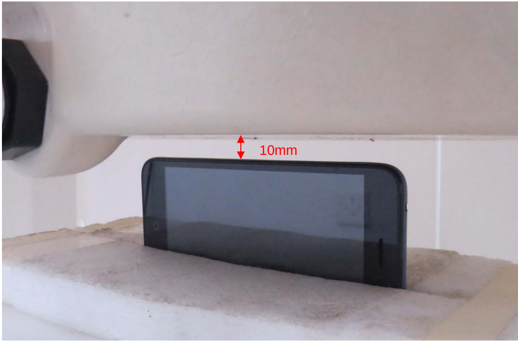
Picture 7: Left Side, the distance from handset to the bottom of the Phantom is 10mm
