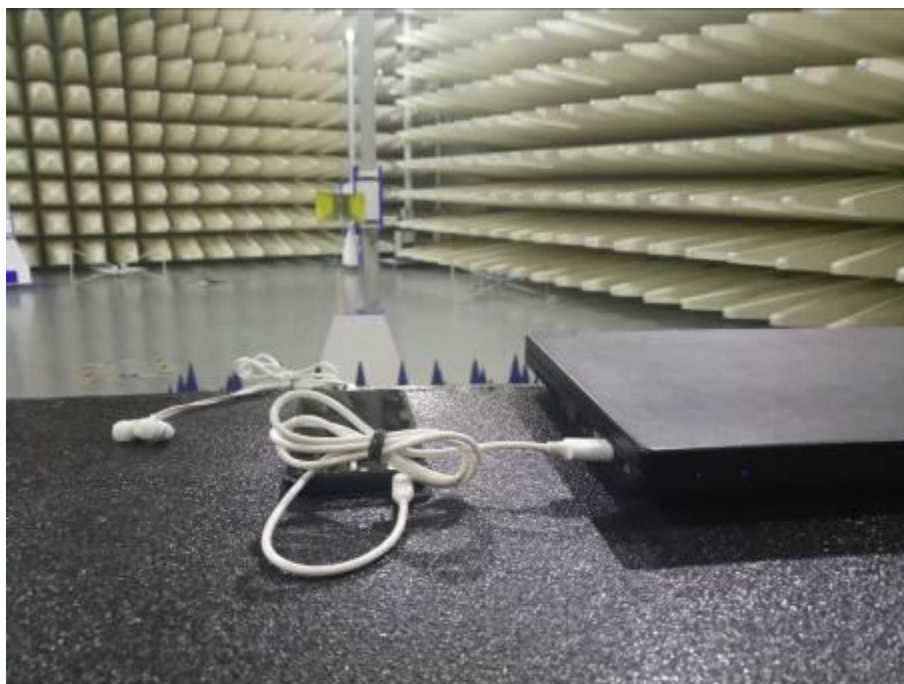
Radiated Emissions Test Setup (with laptop)
