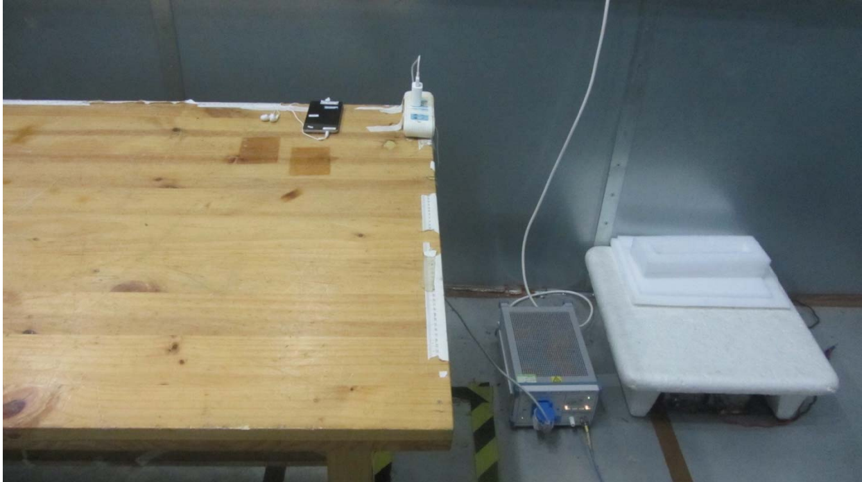
Picture 2 Conducted Emission Test Setup
