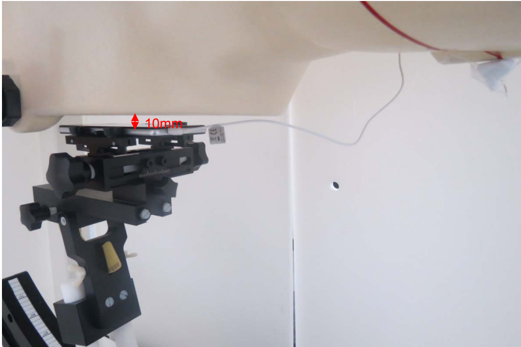
Picture 26: Back Side with Earphone, the distance from handset to the bottom of the Phantom is 10mm
