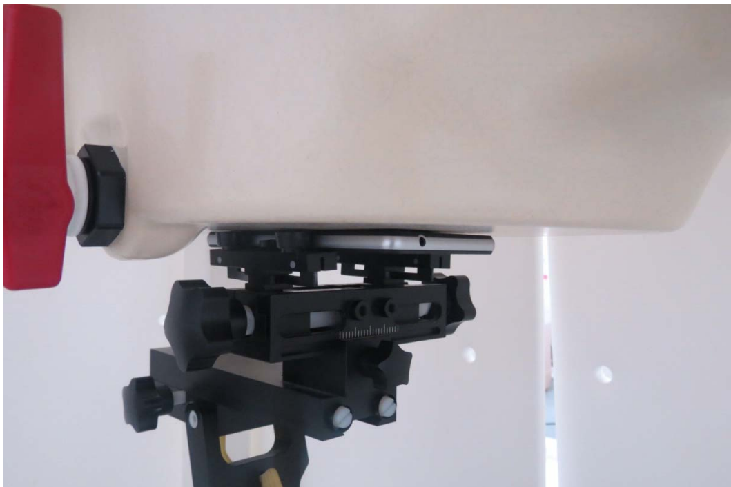
Picture 27: Back Side, the distance from handset to the bottom of the Phantom is 0mm
