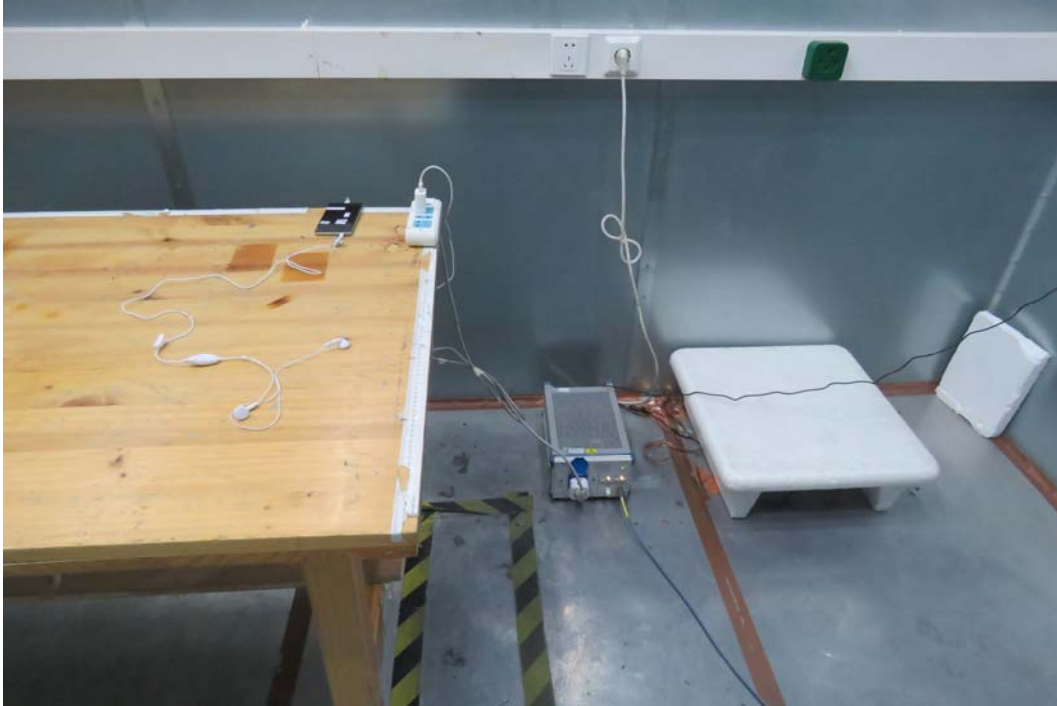
Picture 3 Conducted Emission Test Setup
