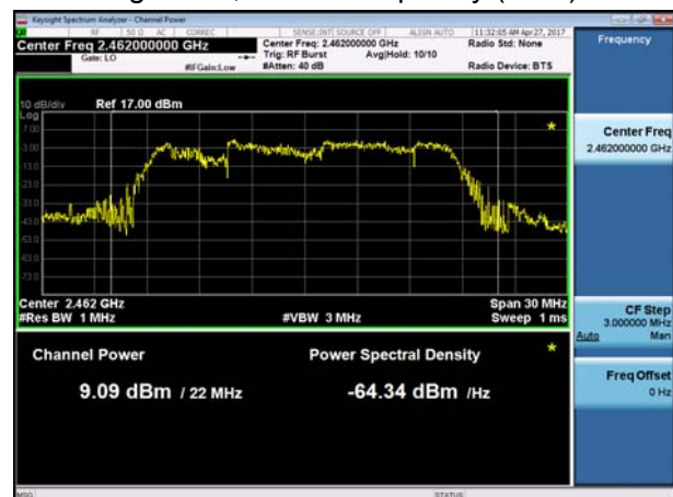
802.11g CH11, Carrier frequency (MHz): 2462
